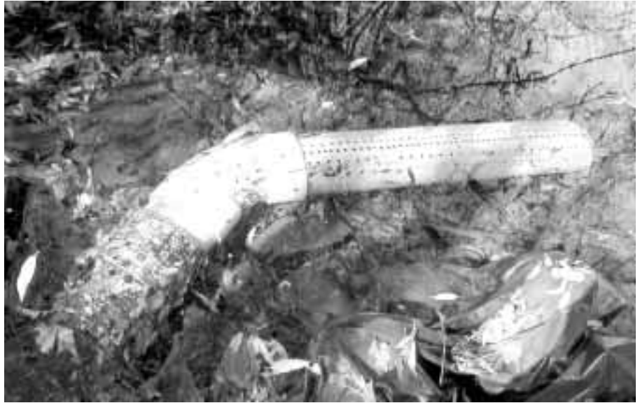
Bob-O's home-built intake made from drilled-out 6 inch PVC pipe.
